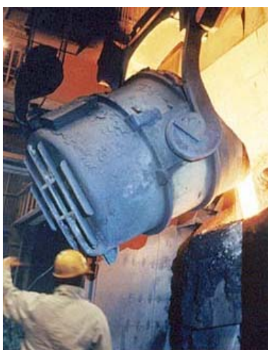
Figure 15. Basic oxygen furnace being charged with molten iron.
